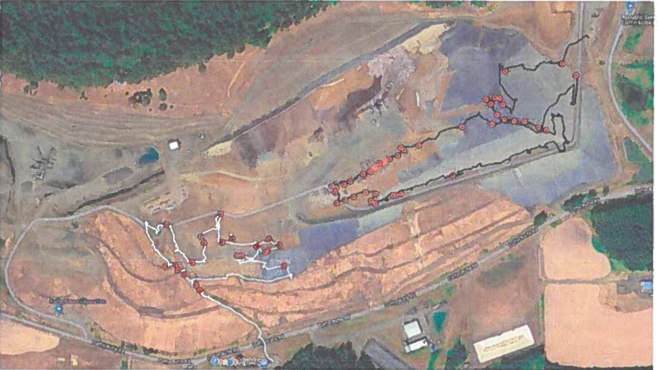
SEM exceedance locations plotted over Google Maps satellite imagery. Approximate monitoring paths included, derived from GPS data. Morning path shown in white, afternoon in black. Line of continuous exceedance at every tarp hole between flags 52 and 54 is highlighted in red.
