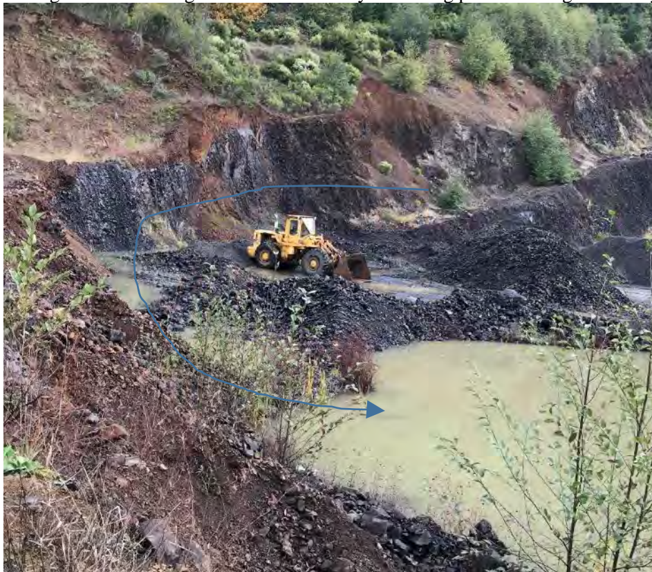
Stormwater along the northern highwall drains westerly to settling pond 1 through a conveyance ditch
