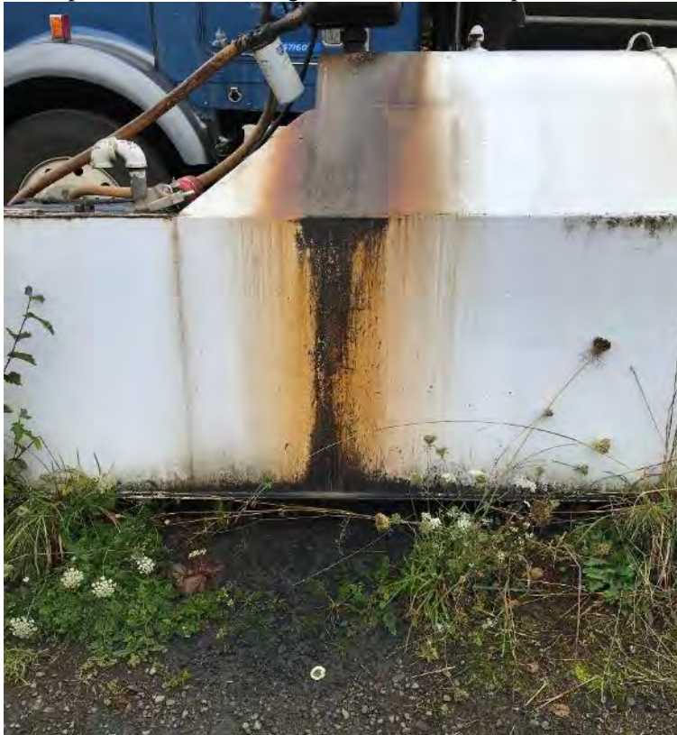
Fuel tank/petroleum stains the ground where it is exposed to stormwater
