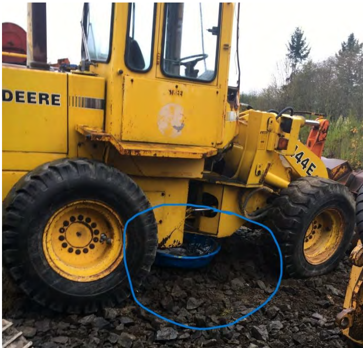
Blue circle represents a secondary containment catch to catch any possible future leaks
